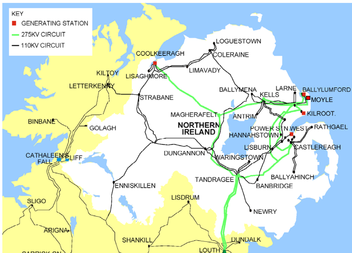
FIGURE 3.1: NIE TRANSMISSION SYSTEM
